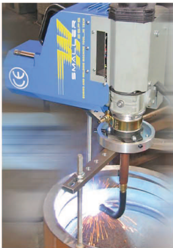
Overlay welding on Ø 380 mm
