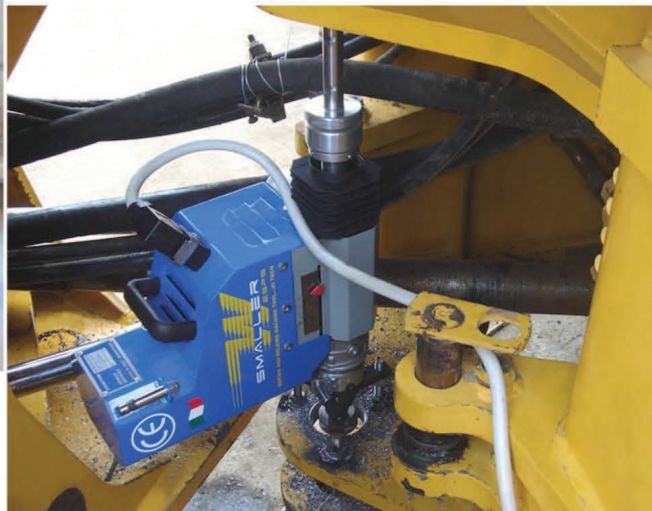
Reconditioning and realignment of the central articulation of a wheel loader. The work is carried out directly on site without disassembling the hydraulic tubes, thus avoiding waste of oil and respecting the environment.
